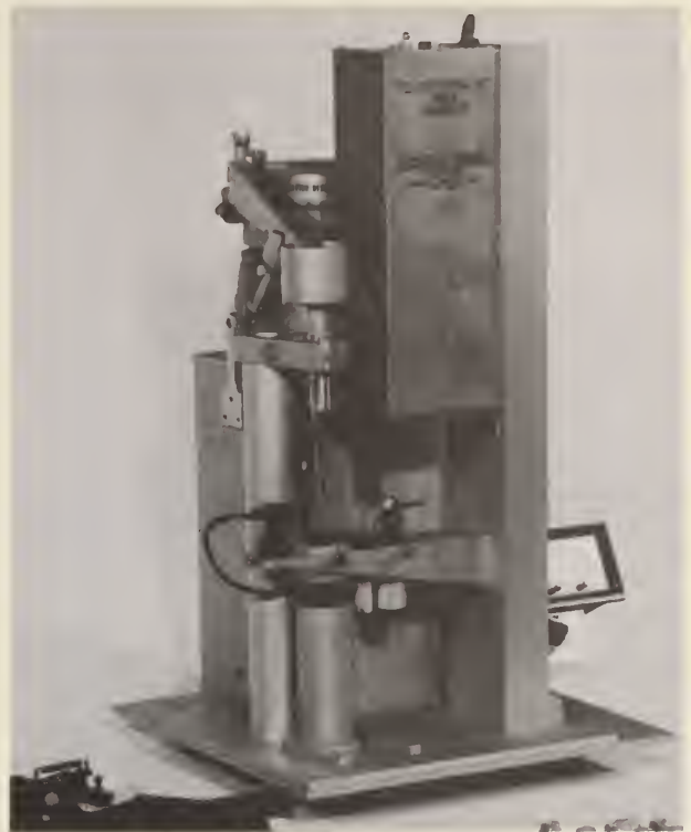
Figure 5 Universal counter designed specifically for small weed seeds using a cheap laser as a collimated light source with beam spreader and collecting lens. Various diameter tapered glass tubes are used to collimate the seed.
